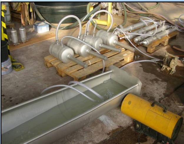
Fig. 1. Equipment destined for work with gases degreased with warm detergent
