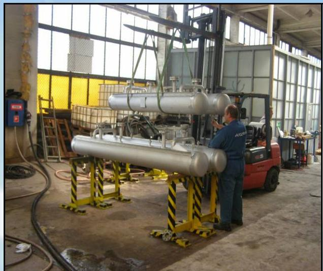
Fig. 3. Preparation of oxygen separators for parallel degreasing
