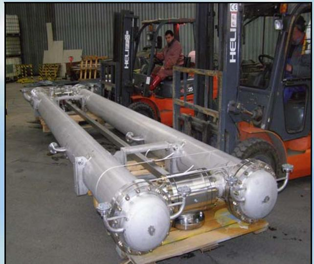
Fig. 6. Oxygen separator after degreasing
