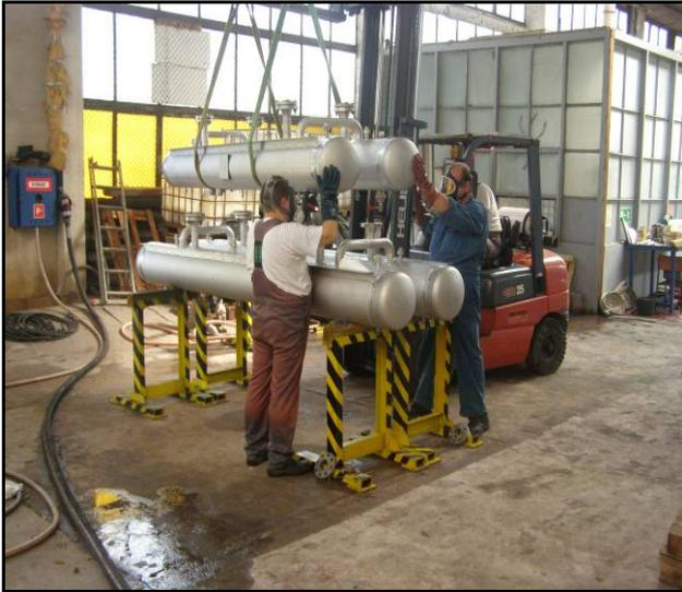
Fig. 4. Consecutive degreasing of oxygen separators
