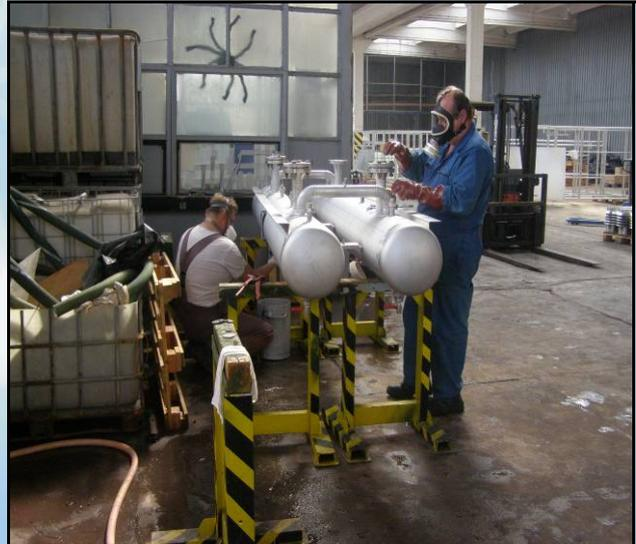
Fig. 2. Degreasing of oxygen separator
