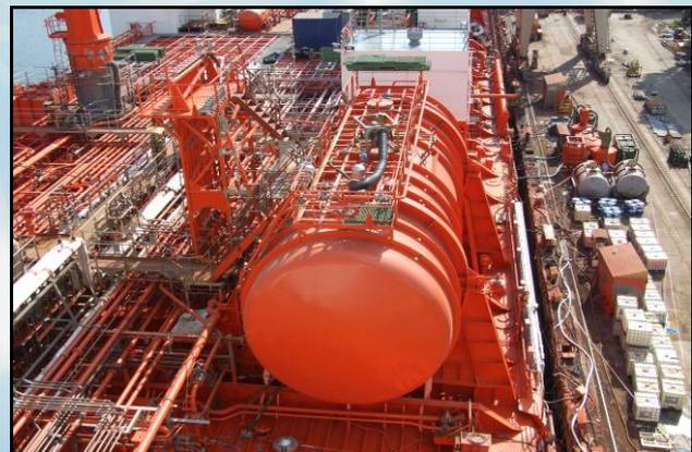
Fig. 3. Slope tanks located over the board
