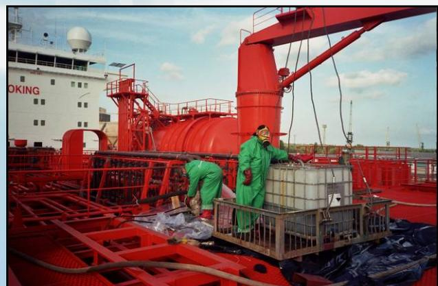
Fig. 5. Chemicals for passivation delivered on the tanker board
