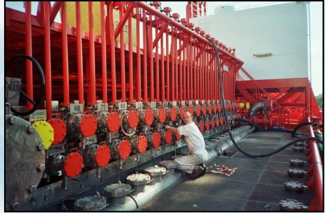
Fig. 8. Flexible temporary connections started from manifold
