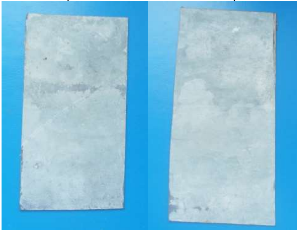
Fig. 14. Galvanized steel plates with lower part immersed in water saturated with poultry meal after 60 days exposure with no corrosion.
