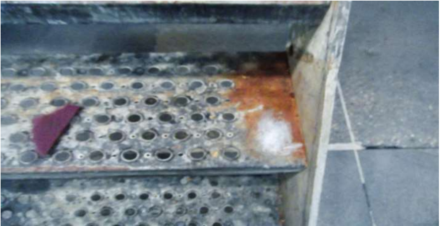
Fig. 3. Coating thickness test performed after removal of strongly adhering deposit showed that zinc film thickness was with no change.
