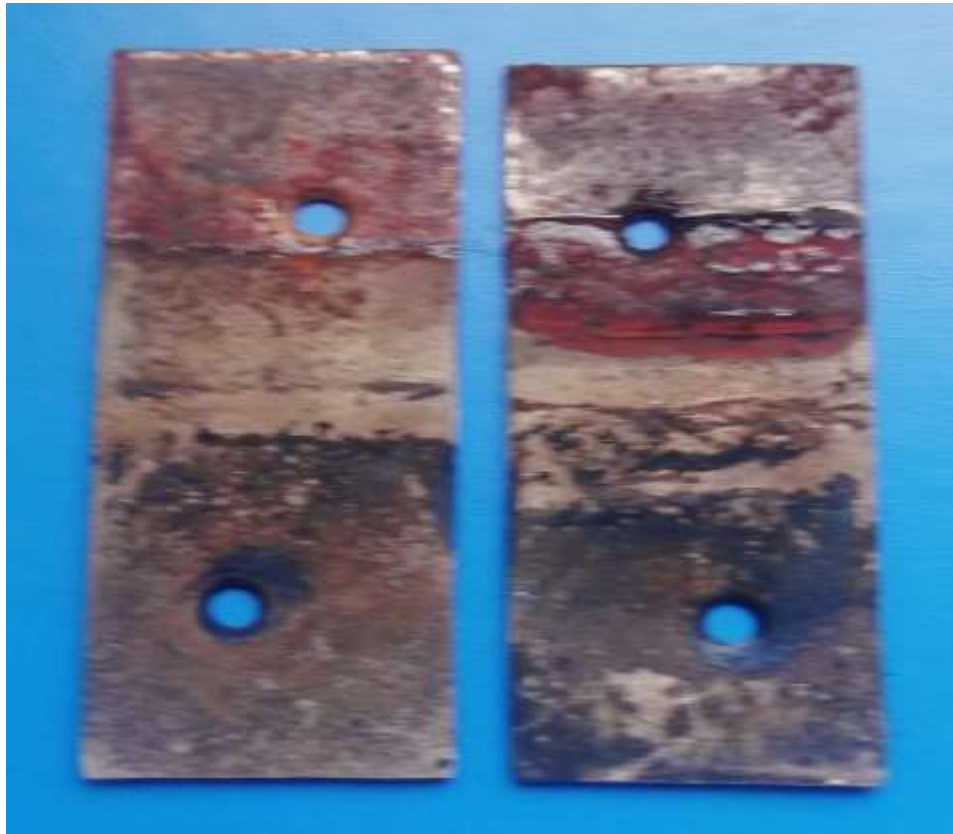
Fig. 13. Steel plates with lower part immersed in water saturated with poultry meal after 50 days exposure. The steel became rusted within vapours above the solution surface. Black deposit on the immersed part.
