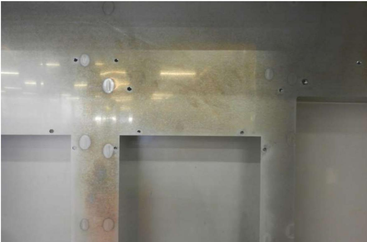
Fig.1. A thin rust film on the construction after storing outdoor. Metallic surface visible on the steel surface after local heat treatment that effected recrystallization
