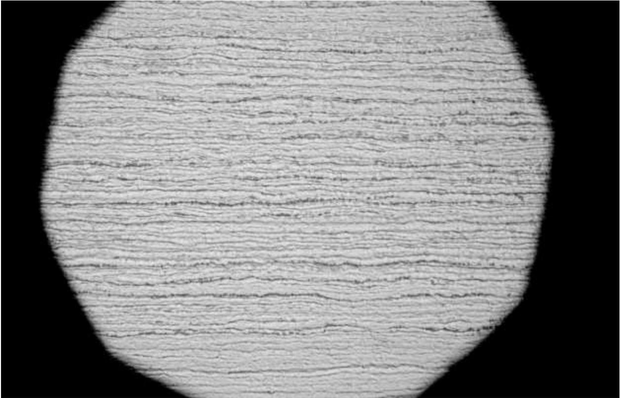
Fig. 3. Fine grained austenite structure of 304 stainless steel with high quantity of parallel thin chains of delta ferrite cells (magnification 500 x)
