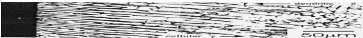
Fig. 4. Microstructure of  $\delta$ -ferrite that may be formed during 304 stainless steel crystallization (Mizukami H, Suzuki T, Umeda T, Kurz W., Mater Sci Eng., 17, 363, 1993.)
