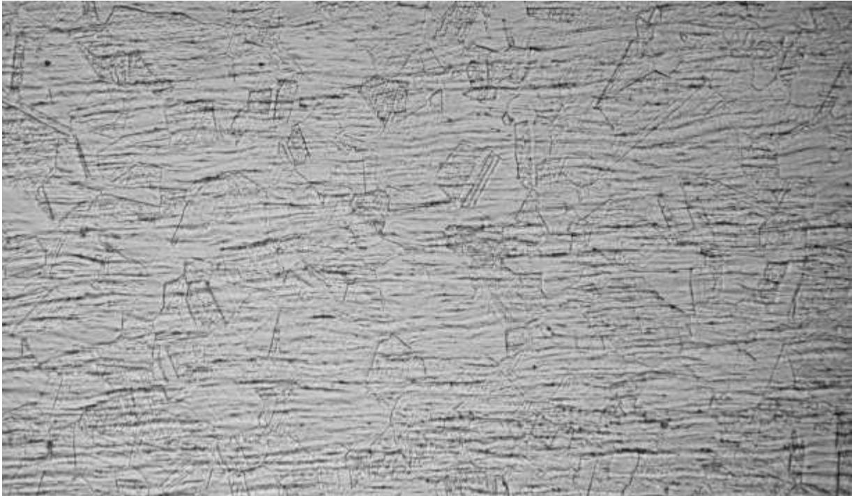
Fig.2. A coarse grained austenite structure of 316 stainless steel that was used traditionally for a production. A tiny presence of ferrite can be found (magnification 400 x)
