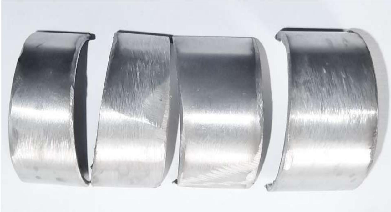
Fig.1. Scratches, local grindings and rust spots present on the external surfaces of the samples
