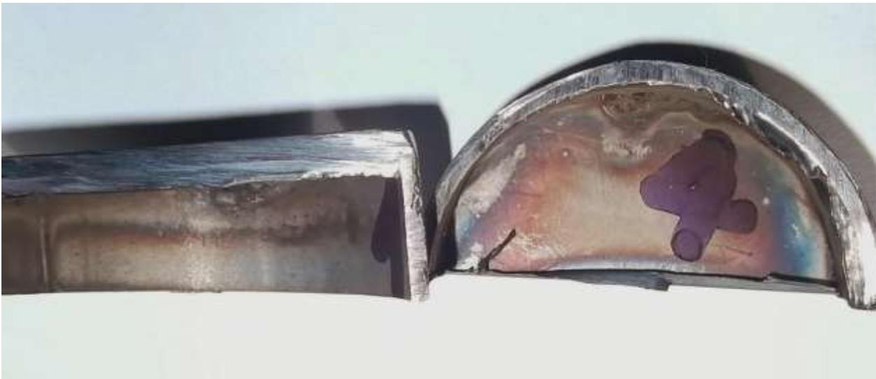
Fig.2. Overwelding was done at some points on welds on internal surface. Grinding marks were present on external surface at places corresponded to the welds
